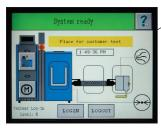
Single-point system operation integrates auxiliary temperature, motor and pressure controls to reduce complexity
